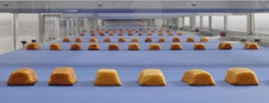
Row distribution system combined with electronic numerical loader for biscuits on edge
